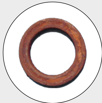
Suspension bearing corroded due to ingress of contaminants
