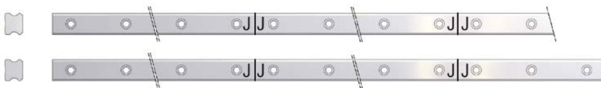
Figure 3.6 Marking of jointed rails
