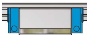
Overhead installation, rotation by 180° y - 180°
