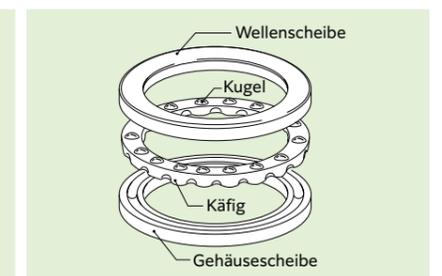
Abb. 5.6 Axialkugellager
