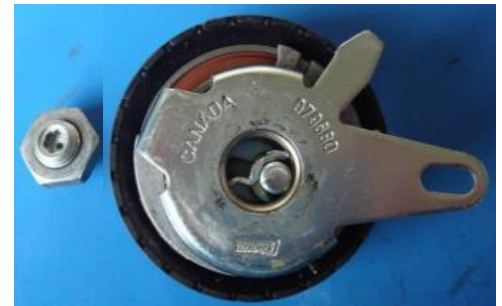
Roller GT357.28 with broken shaft
