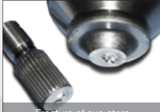
Fracture of cup stem
