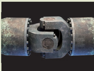
Photo showing condition of U-joint after operation
