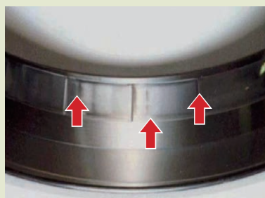
Excessive wear occurred
